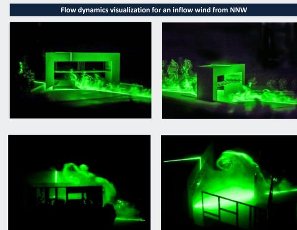
Turbulent vortices within the audience area, for the **reference scenario (above)**, and the **mitigation scenario (below)**. In the latter, the vortices are driven over the portico due to the presence of the front panels.
