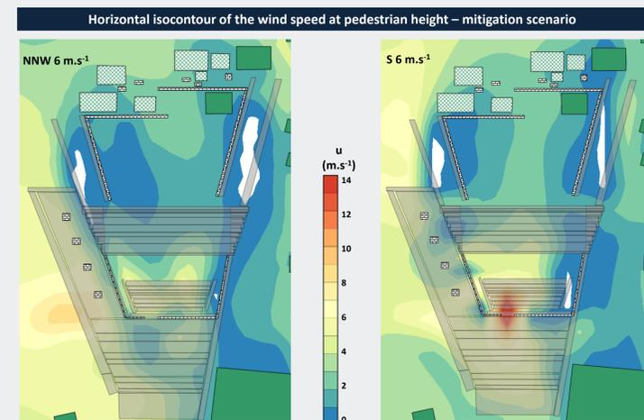
The results show a reduction of wind speed between 4 and 6 m.s<sup>-1</sup> within the auditorium, with the mitigation measures. There is also an attenuation in recirculation near the wall, upstream from the auditorium, leading to an effective reduction of the wind speed.
