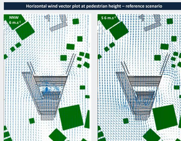
In front of the auditorium, the turbulent flow is channelled with an increase of wind speed, due to its configuration. The highest wind speeds are mainly simulated in the audience area.
