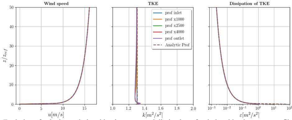
**Figure 2.** Evolution of velocity, turbulent kinetic energy and dissipation of turbulent kinetic energy profiles along 2D domain of 5 km and with  $z_{ref}$  of 6 m. The ground wall function uses a Hargreaves and Wright, (2007) correction.
