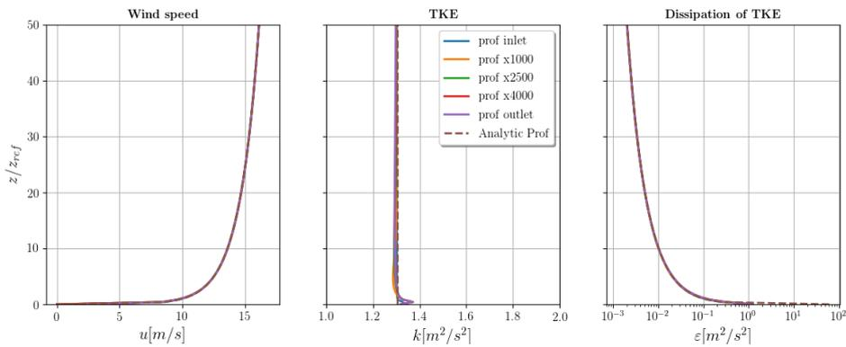
**Figure 1.** Evolution of velocity, turbulent kinetic energy and dissipation of turbulent kinetic energy profiles along 2D domain of 5 km and with  $z_{ref}$  of 6 m. Overall setting: Hargreaves and Wright, (2007). The intermediate profiles are at 1 km, 2.5 km and 4 km. The ground wall function uses a standard roughness model, available in OpenFOAM.
