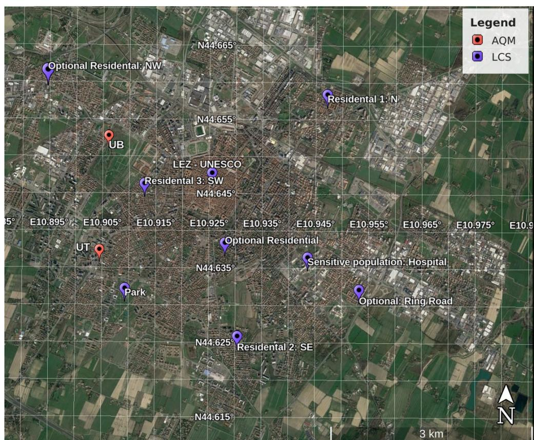
**Figure 1.** Preliminary map of the low-cost sensor network for Modena. AQM red marks indicate regulatory Air Quality Monitoring stations. LCS purple marks indicate the location of the low cost sensors.
