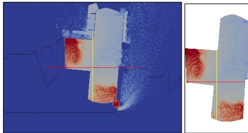
**Figure 4,** Ground concentration computed in the Grand Palais nested domain (left hand side) and close-up view of the largest room (right hand side). Concentrations are ranging from low values (blue) to large values (red)
