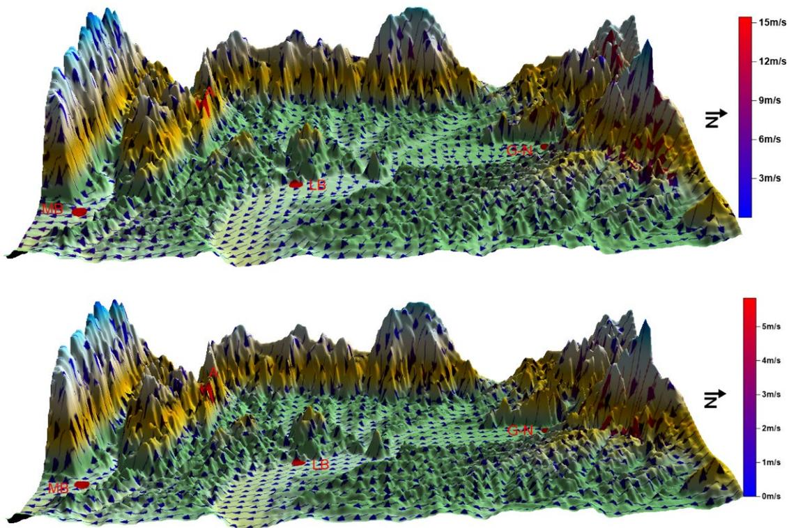
**Figure 4.** Local flow fields with WRF-GRAMM initialisation (top) and WRF/monitoring initialisation (bottom).
