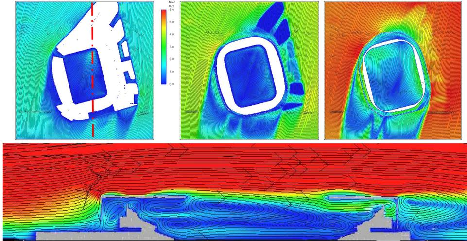
**Figure 4.** Horizontal and vertical cuts of the wind field on domain N03. The horizontal cuts are represented at a height of 4 m (middle of the lower rostrum), 13 m (middle of the intermediate stand) and 21 m (middle of the upper stand). The vertical section plane is indicated by the red line on the first illustration.
