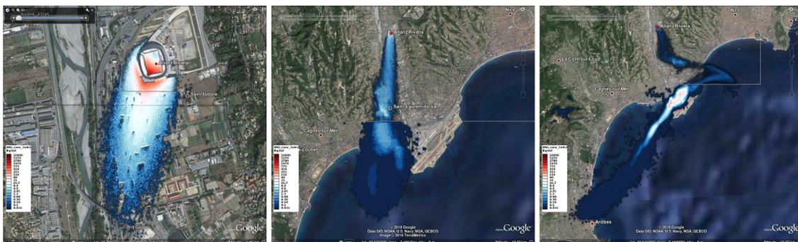
**Figure 5.** Concentration field after the release at different time frames (4 min, 30 min and 80 min, left to right).
