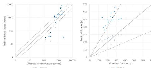
**Figure 4.** CUTE wind tunnel puff releases. Scatter plot of the predicted and measured mean dosage (left) and mean duration (right), for MSS (asterisks) and PMSS\_D (circles).
