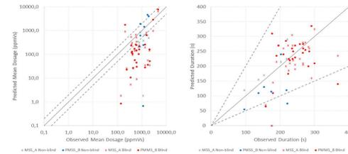
**Figure 2.** Michelstadt puff releases. Scatter plots of the predicted and measured mean dosages (left) and puff mean durations (right), for the non-blind test cases (S2, S4 and S5 sources, blue colour) and the blind test cases (S5, S6, S7 and S8 sources, red colour) for MSS\_A (asterisks) and PMSS\_B (circles) configurations.
