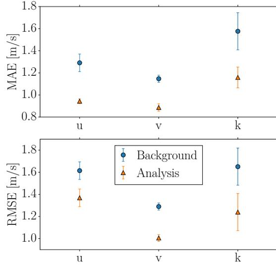
**Figure 4:** Mean absolute error (MAE, above) and root mean square error (RMSE) of the simulated wind components ( $u$  and  $v$ ) and turbulent kinetic energy ( $k$ ), before (blue) and after (orange) the analysis cycle of the IEnKS. The errorbars show the standard deviation of the background and analysis ensembles for the MAE and the RMSE.
