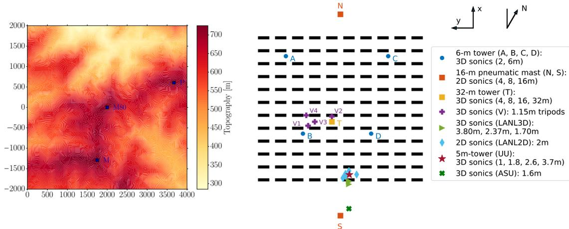
**Figure 2:** (left) Topography for the domain used in the first experiment and location of the three meteorological masts (blue squares). (right) Representation of the *Code\_Saturne* domain containing the MUST array with the location of the available meteorological instruments.
