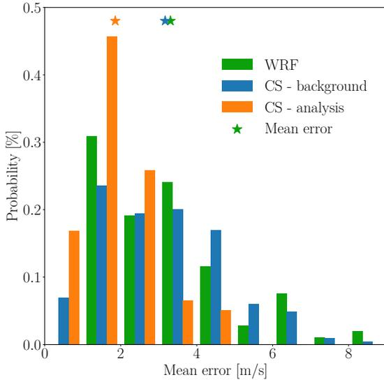
**Figure 3:** Histograms of the errors between sonic observations, provided by the mast M80, and the wind simulated by WRF (green), by *Code\_Saturne* with BCs provided by WRF (background, blue), and by *Code\_Saturne* with BCs corrected by the IEnKS (analysis, orange). The mean error made by WRF (green), *Code\_Saturne* before (blue) and after (orange) DA are also shown (stars).
