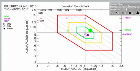
**diamond diagram:** it is designed to identify discrepancies between inventories; it allows to assess whether the differences can be mostly related to different emission factors or in the choice of activity data
