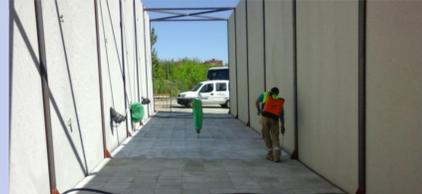
The photocatalytic material (coating) was only applied on the tiles of one of the streets, "photoactive street" (3<sup>rd</sup> May 2016). The NO depolluting efficiency was 65% under the ISO international standard [2].
