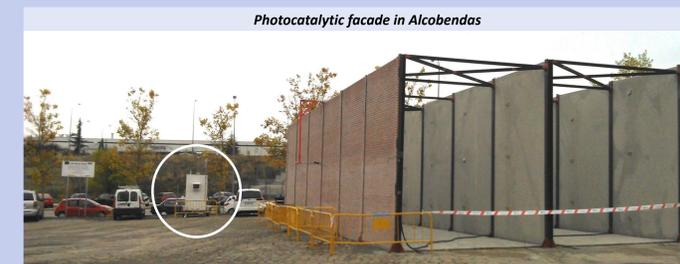
A mobile monitoring station (marked in the image) was installed near the street canyon for the continuous measurement of NO, NO<sub>2</sub> and O<sub>3</sub> concentrations and meteorological parameters in both scenarios measurement in order to document the evolution of the physical chemical characteristics of the air mass existing in the zone and obtain fundamental information for a correct interpretation of the results.
