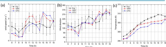
Figure 3. Time series of the experimental data, WRF and CFD results of: (a) wind speed, (b) wind direction and (c) temperature at 18 m AGL (yellow point in Fig. 1).
