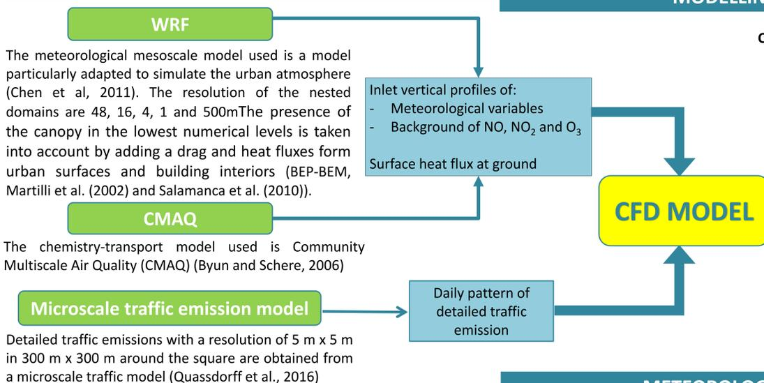
CFD model based on the Reynolds-averaged Navier-Stokes (RANS) equations with the realizable turbulence k-ε closure
