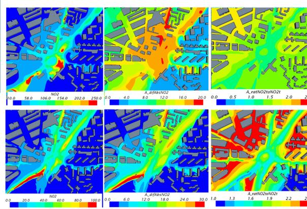
Figure 8. (left to right) The spatial distribution of NO<sub>2</sub> concentration (ppb), NO<sub>2R</sub>-NO<sub>2T</sub> and the ratio NO<sub>2R</sub>-NO<sub>2T</sub> at (above) 06UTC and (below) 12UTC.
