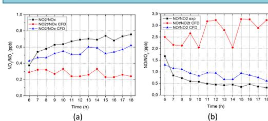
Figure 7. Time series of: (a) NO-to-NO<sub>2</sub> and (b) NO<sub>2</sub>-to-NO, registered at air quality monitoring station (black) and the CFD results by simulating the pollutants as inert species (red) and reactive compounds (blue)
