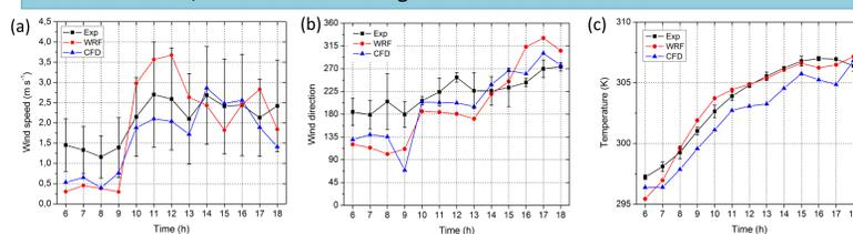
Figure 4. Time series of experimental data, WRF and CFD results of: (a) wind speed, (b) wind direction and (c) temperature at 8 m AGL (blue point in Fig. 1)
