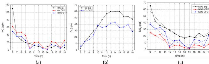
Figure 6. Time series of: (a) NO, (b) O<sub>3</sub> and (c) NO<sub>2</sub> concentrations in ppb registered at air quality monitoring station (black) and the CFD results by simulating the pollutants as inert species (red) and reactive compounds (blue)
