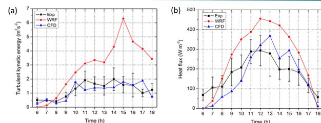
Figure 5. Time series of WRF and CFD results against to the experimental data of: (a) HF and (b) k
