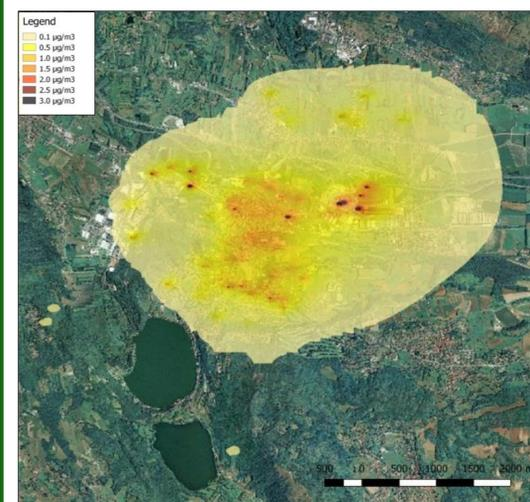
The figure shows the results obtained through the modeling of the emission scenario determined by the substitution of the whole traditional fuel heating network with wood biomass boilers.
