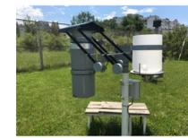
Automatic samplers for wet and dry deposition (WADOS - Kroneis GmbH)
