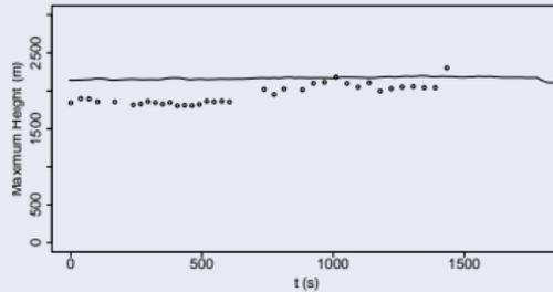
Mean plume height: model vs observations, New plume rise scheme
