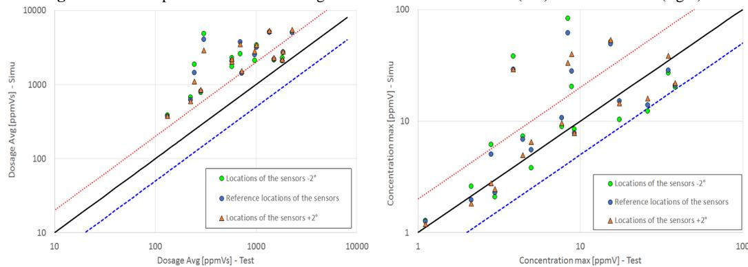
**Figure 6:** Scatter plots of the mean dosage (left) and peak concentration (right) for CASE3-puff.
