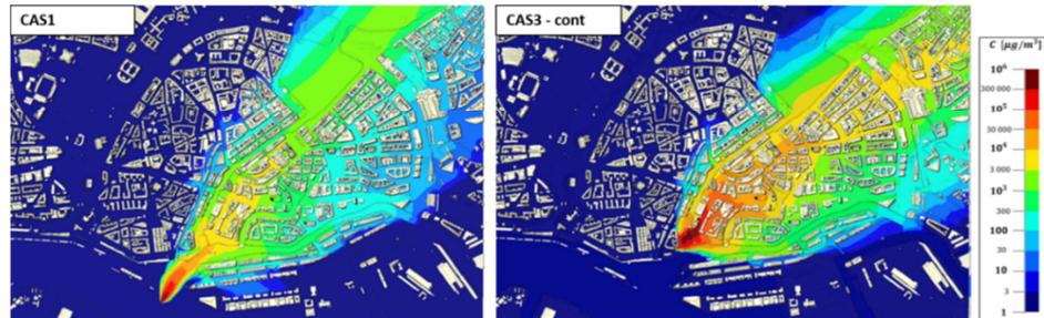
**Figure 3:** CASE1 and CASE3-continuous – Time-averaged concentration field at 2 m above the ground level.
