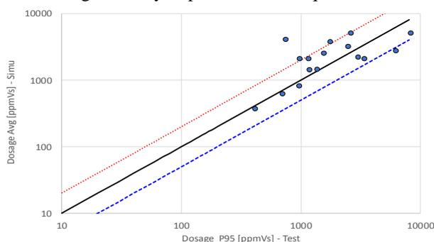
**Figure 7:** Scatter plot of the 95<sup>th</sup> percentile dosage for CASE3-puff.
