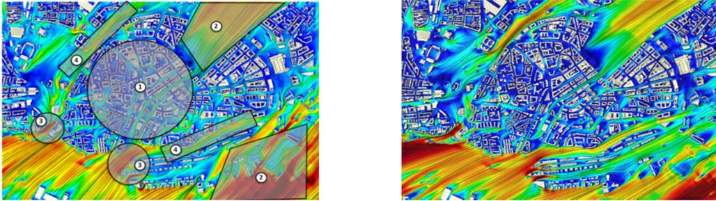
**Figure 2:** Time-averaged velocity at 10 m above the ground level. Left: CASE1 with zone definition, Right: CASE3.
