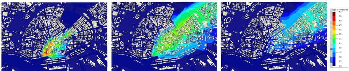
**Figure 4:** CASE3-puff – Averaged concentration field (over 5 minutes) at 2 m above the ground level. Left: 0-5 minutes, centre: 10-15 minutes, right: 25-30 minutes.
