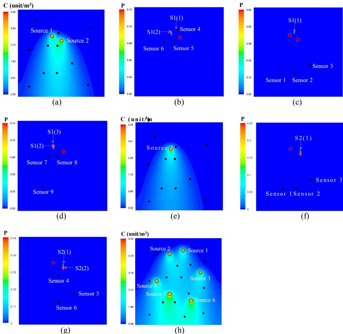
Figure 3. Identification of multiple pollutant sources in an open space: (a) “Actual” condition with two sources; (b) The first trial for S1 get S1(1); (c) The second trial for S1 gets S1(2); (d) The third trial for S1 gets S1(3); (e) Simulated pollution field by Source 1 (f) The first trial for S2 gets S2(1); (g) The second trial for S2 gets S2(2); (h) Case with six pollutant sources.
