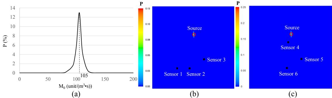
Figure 2. Identification of single pollutant source: (a) Largest probability corresponding different assumed source strength; (b) The first trial to identify the source; (c) The second trial to identify the source
