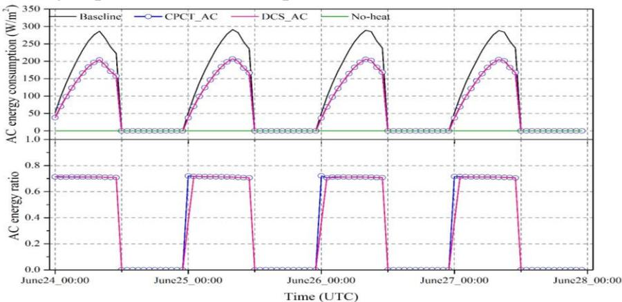
Figure 3. Comparison of air-conditioning energy consumption in the non-domestic areas for different cases.
