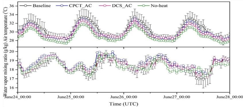
**Figure 1. Comparison of mean 2-m air temperature and water vapor mixing ratio in non-domestic areas in the commercial areas for the baseline case, CPCT\_AC case, DCS\_AC case, and no-heat case**
