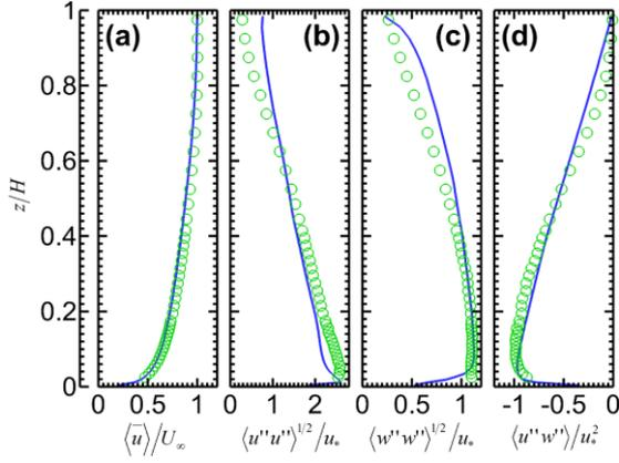
**Figure 2:** Vertical profiles of (a) mean wind speed; (b) streamwise fluctuating velocity; (c) vertical fluctuating velocity and (d) vertical momentum flux. Solid line: LES data and symbols: wind tunnel data (Ho and Liu 2016).
