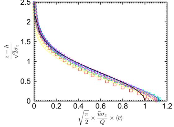
**Figure 3:** Profiles of dimensionless concentration of passive scalar at  $x/h =$ : (a) 15.5 ( $\square$ ), (b) 25.5 ( $\triangle$ ), (c) 35.5 ( $\nabla$ ), (d) 45.5 ( $\triangleright$ ), (e) 55.5 ( $\triangleleft$ ) and (f) 65.5 ( $\diamond$ ). Theoretical Gaussian plume profile (—)
