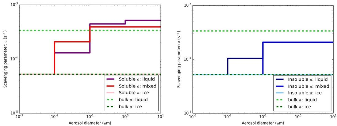
**Figure 2.** Variation of in-cloud scavenging parameter  $a$  with particle diameter in liquid, mixed and ice phase clouds for soluble (left) and insoluble (right). For comparison, the in-cloud bulk scavenging parameters used by default in NAME are shown.
