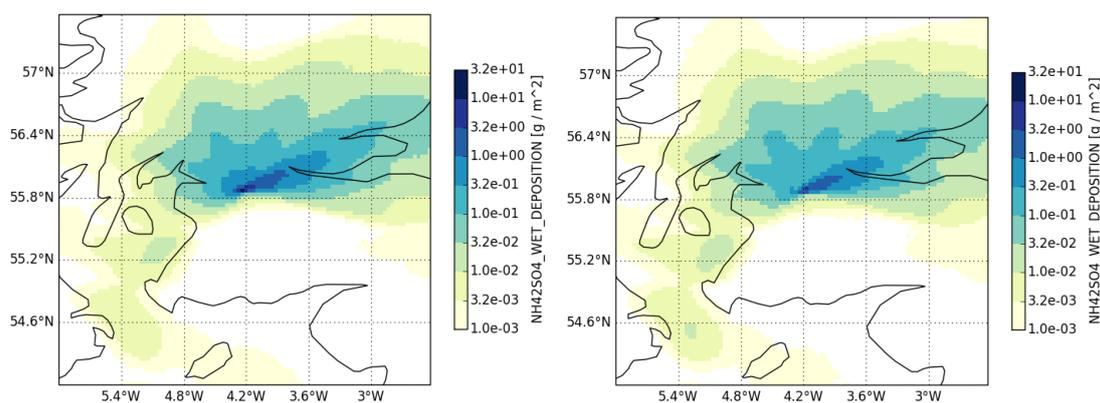
**Figure 3.** A comparison of NAME predicted total wet deposition of  $(\text{NH}_4)_2\text{SO}_4$  obtained using the bulk wet scavenging scheme (left) and the new particle size dependent wet deposition scheme (right).
