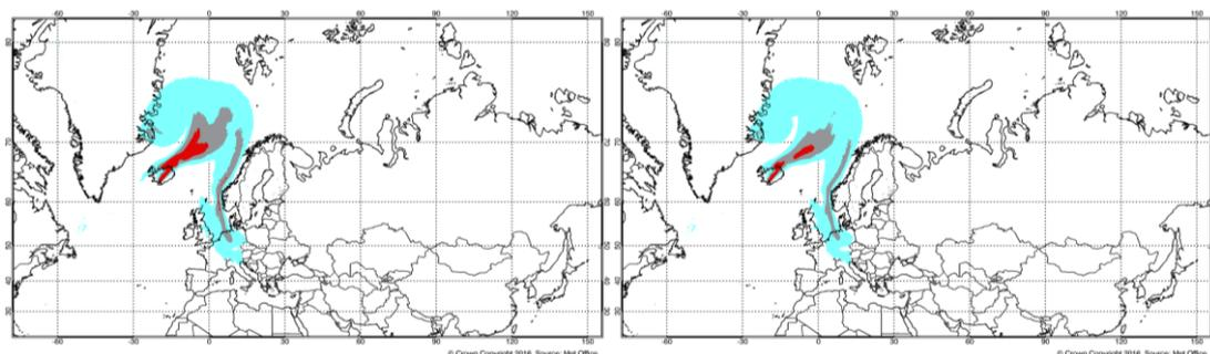
**Figure 4.** A comparison of NAME predicted 6-hourly averaged ash concentrations from the eruption of Eyjafjallajökull in 2010 using the bulk wet scavenging scheme (left) and the new particle size dependent wet deposition scheme (right). Ash concentrations between 12:00 - 18:00 UTC on 18/05/2012 and from FL000 - FL200 are shown in three concentration ranges: 200 - 2000  $\mu\text{g m}^{-3}$  (cyan), 2000 - 4000  $\mu\text{g m}^{-3}$  (grey) and  $> 4000 \mu\text{g m}^{-3}$  (red).
