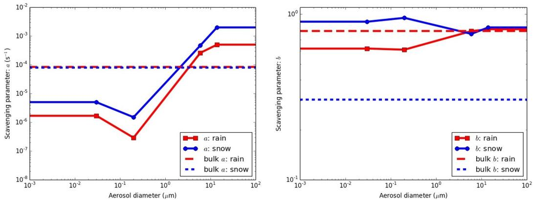
**Figure 1.** Variation of below-cloud scavenging parameters,  $a$  (left) and  $b$  (right), with particle diameter. For comparison, the bulk scavenging parameters used by default in NAME are shown.
