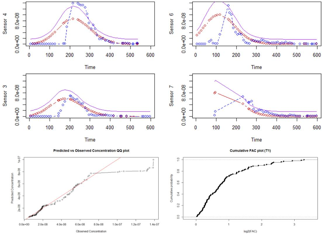
**Figure 1.** Predicted traces for the four maximally responding sensors (top – blue: measured; red: model; solid line: model plus standard deviation) and QQ and CF summary plots (bottom) for JU2003 puff release IOP3 R3.
