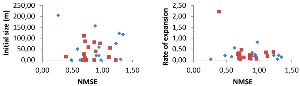
**Figure 2.** Left: plot of  $\sigma_{x0}$  against NMSE for each puff release in the JU2003 trial. Right: plot of the expansion rate  $\gamma$  against NMSE for each puff release in the JU2003 trial. Blue markers: daytime; red: night.
