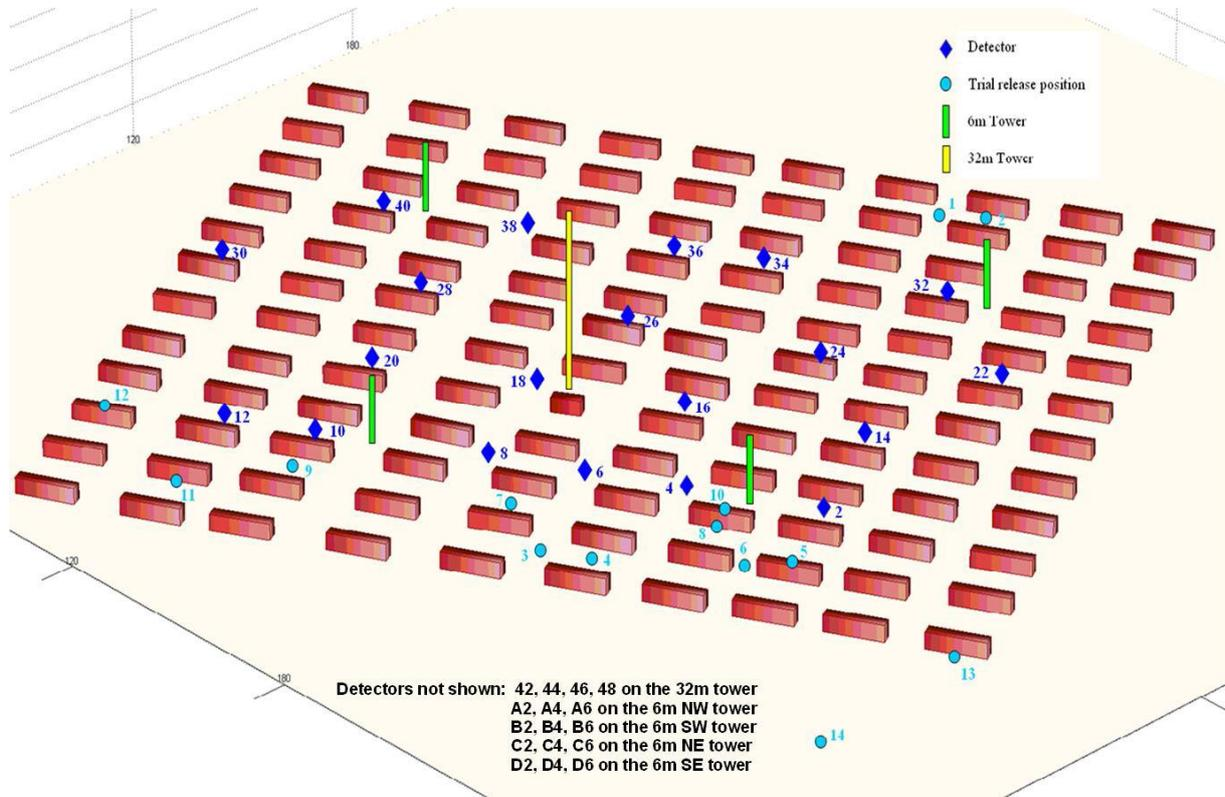
**Figure 1.** MUST Trials Setup Showing the Release Locations and Detector and Met Tower Positions
