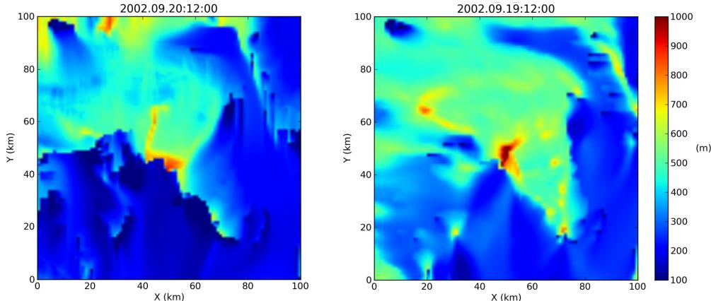
**Figure 5.** Spatial distribution of the simulated mixing height for 20/9/2020 12:00 LST (left) and 19/9/2020 12:00 LST (right) calculated using the B4 and B4f model configurations, respectively
