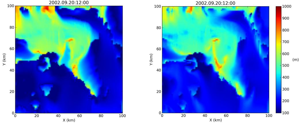
**Figure 3.** Spatial distribution of the simulated mixing height for 20/9/2002 12:00 LST calculated using the A1 (left) and B1 (right) model configurations
