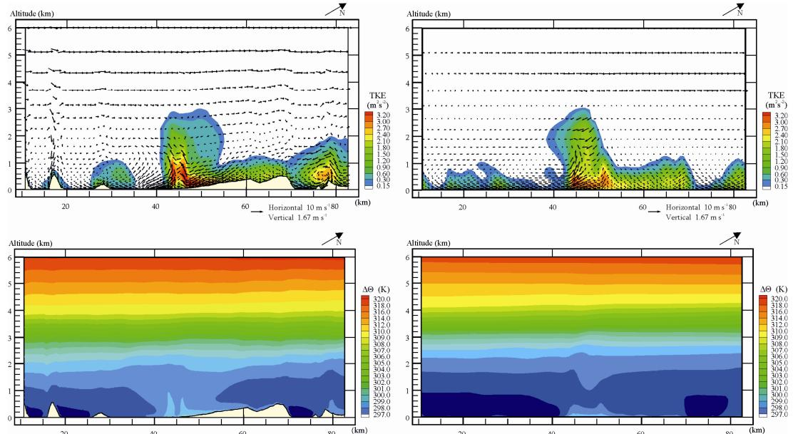
**Figure 4.** Vertical section of TKE (top) and potential temperature (bottom) calculated for 20/9/2002 12:00 LST with the B4 (left) and for 19/9/2002 12:00 LST with the B4f flat-topography (right) configurations. The section plane is parallel to the NNE-SSW direction.
