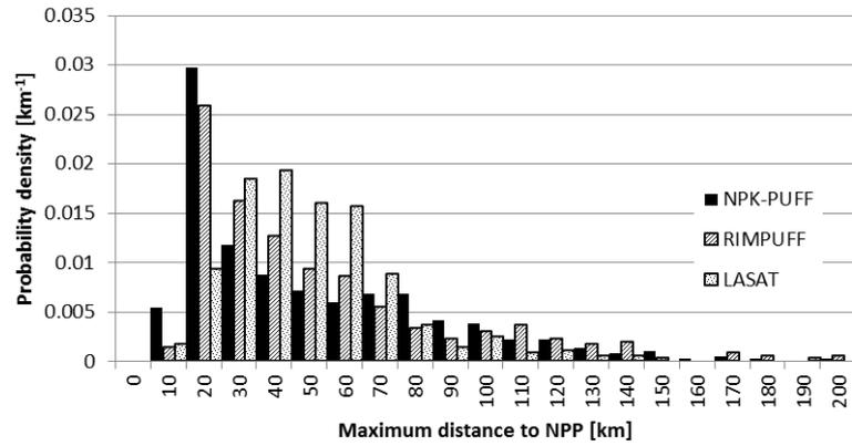
Figure 1: Probability density of maximum distance to the nuclear power plant (NPP) where  $TIAC_{crit}$  is reached.
