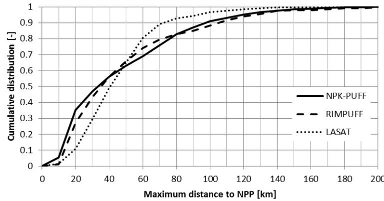
Figure 2: Cumulative distribution of maximum distance to the nuclear power plant (NPP) where  $TIAC_{crit}$  is reached
