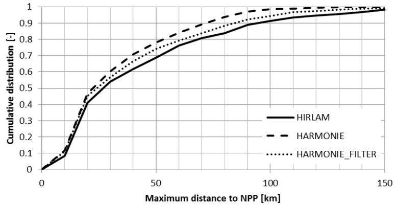
Figure 3: Cumulative distribution of maximum distance to the nuclear power plant (NPP) where TIACcrit is reached
