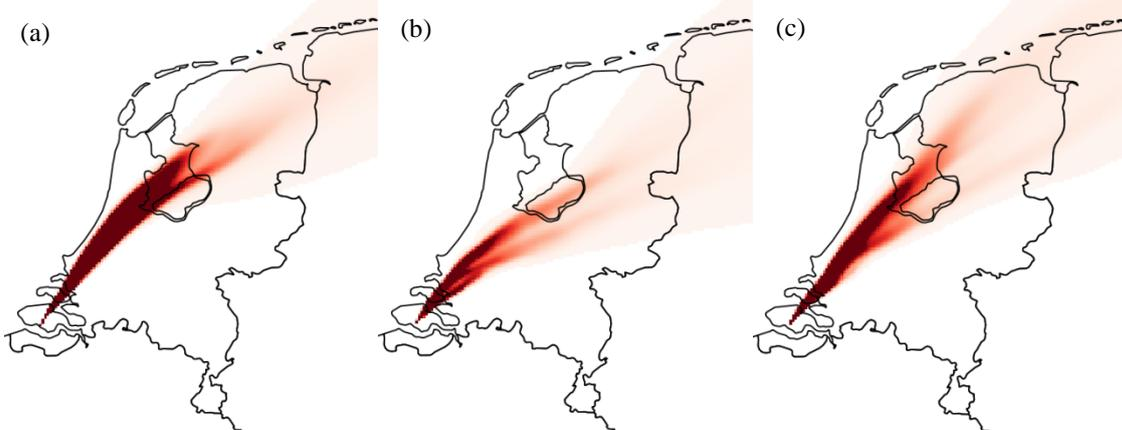
Figure 5: Release on April 11 2015 at 20:00 (UTC) from NPP Borssele modelled with NPK-PUFF. Air concentration integrated over 48 hours. Using a) HIRLAM. b) HARMONIE. c) HARMONIE with filtered mixing height data.
