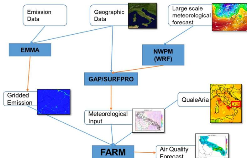
**Figure 1.** Schematic representation of AQFS.
