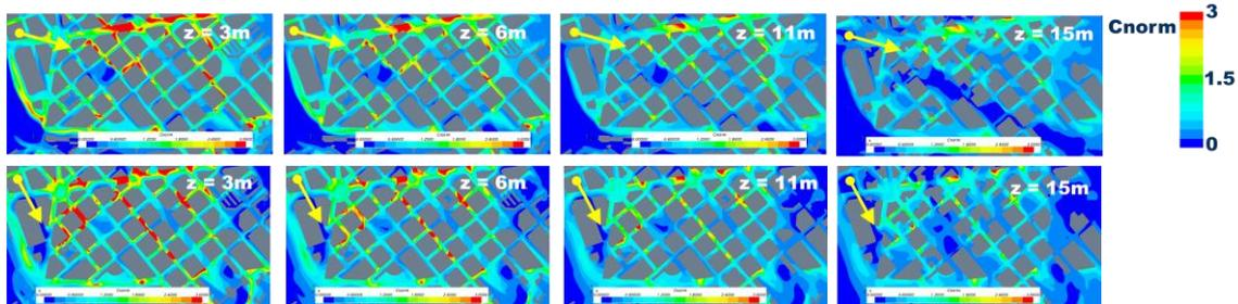
**Figure 5.** Normalized concentration at different heights above ground level (AGL) for WNW and NWN wind directions (above and below panels, respectively).
