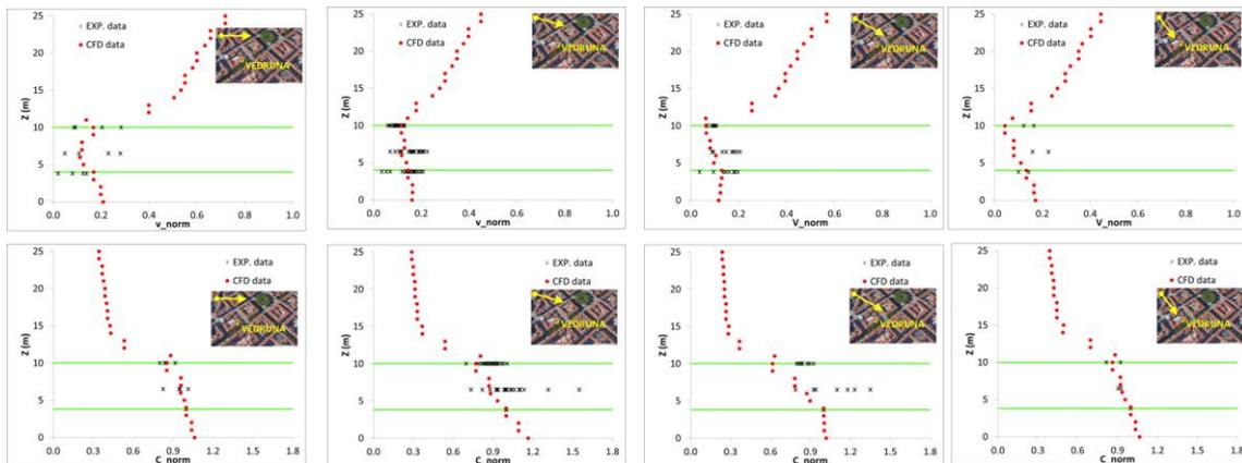
**Figure 3.** Experimental and modelled vertical profiles of normalized horizontal wind speed (top panels) and BC concentrations (bottom panels) for different inlet wind directions in the street with trees.
