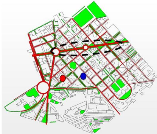
**Figure 2.** Numerical domain. Green represents vegetation and red traffic emission zones. Red point: Vedruna location (street with trees); Blue point: PC location (street without trees)
