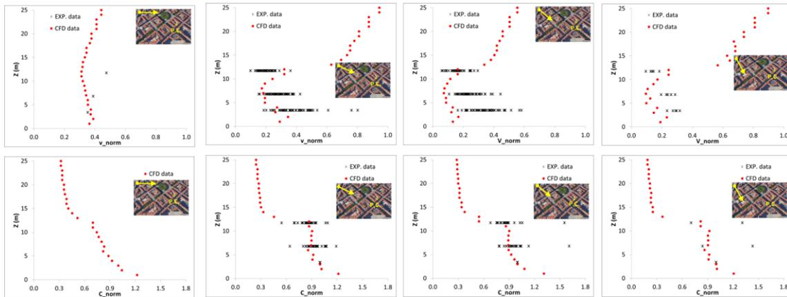
**Figure 4.** Experimental and modelled vertical profiles of normalized horizontal wind speed (top panels) and BC concentrations (bottom panels) for different inlet wind directions in the street without trees.
