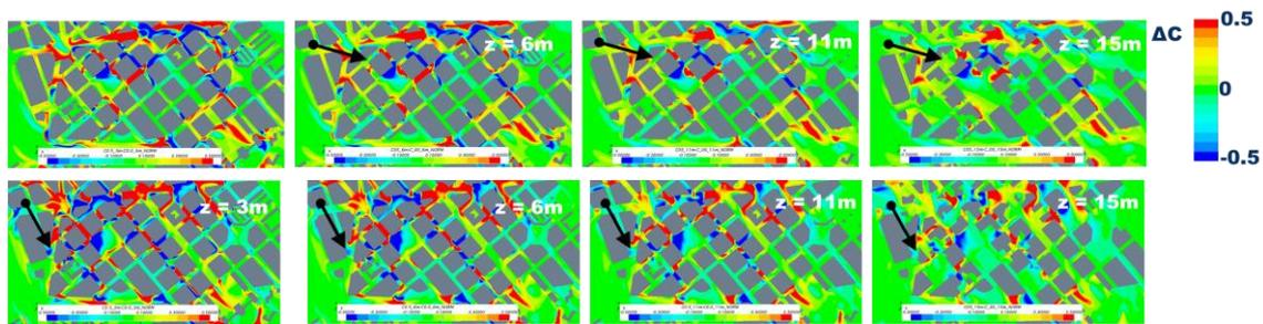
**Figure 6.** Differences of normalized concentration at different heights AGL between a simulation considering the aerodynamic effects of vegetation (no deposition) and a simulation without any vegetation in the domain for inlet wind direction from WNW (above) and NNW (below).
