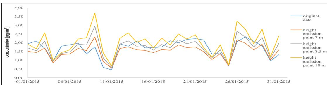
**Figure 3.** Average concentration trend at varying the height of emission point in correspondence of a receptors
