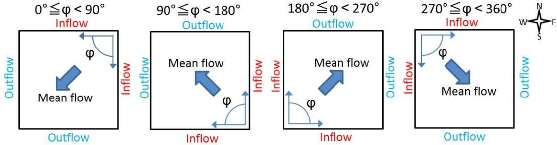
**Figure 2.** Schematic of the treatment of inflow and outflow boundaries depending on different mean wind directions.
