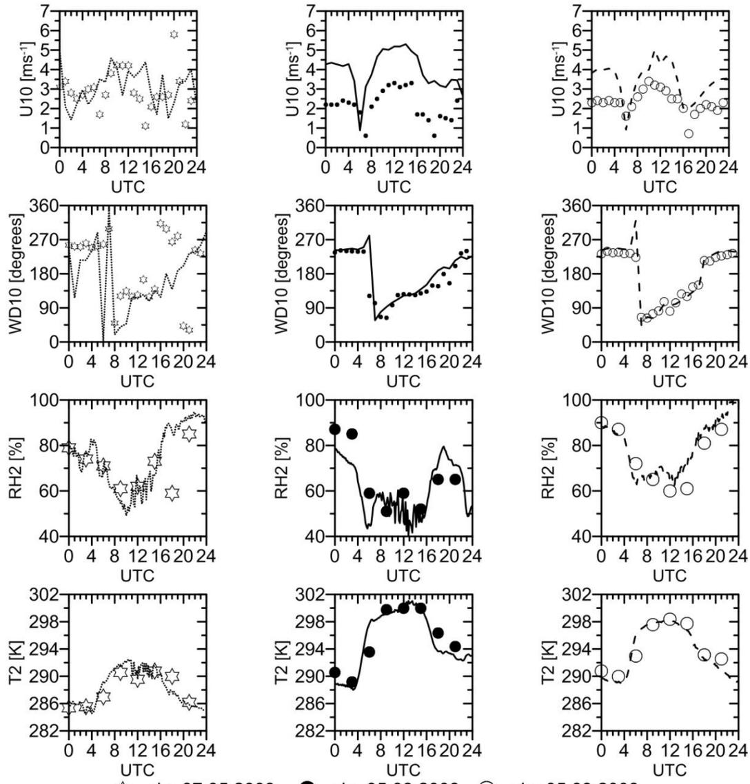
**Figure 2 a.** Comparison between modelled (output at every 1h) and measured (at every 3 h)  $T2$ ,  $RH2$  at Ahtopol station.  $U10$  and  $WD10$  were measured (at every 1 h) by automatic anemometer MS&E – Wind2
