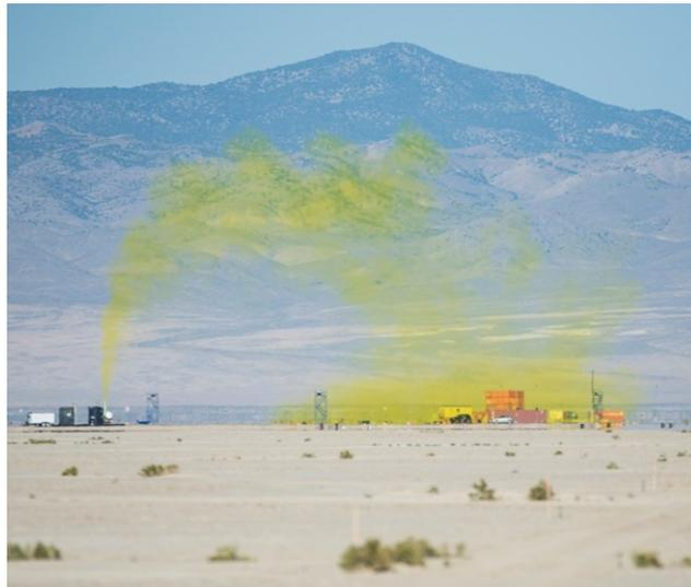
**Figure 3.** Photo of JR II Trial 8 dense jet plume about 30 s after the release initiated. The distance from the source tank to the tall red obstacle is about 85 m.
