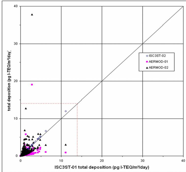
**Figure 1.** Scatterplots of total deposition results obtained with AERMOD and ISC3ST simulations. The dashed line indicates the reference value adopted (14 pg I-TEQ/m²/day).
