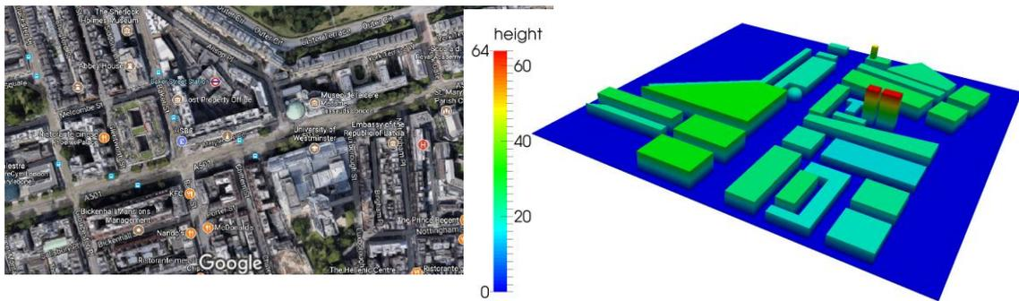
**Figure 1.** Overview of Marylebone Rd and surrounding area (left). Schematic of the area used for computation (right). The colour scheme indicates the building heights in meters. The image is taken from Municchi (2014).
