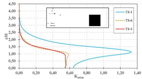
Figure 8. Dispersion profiles downstream of the building.
