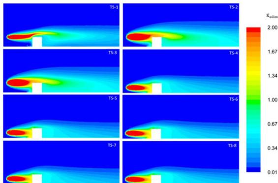
Figure 7. Contour of dispersion field,  $K_{adim}$ , view of the symmetry plan of the building for the sensitivity tests (TS-1) - (TS-8)
