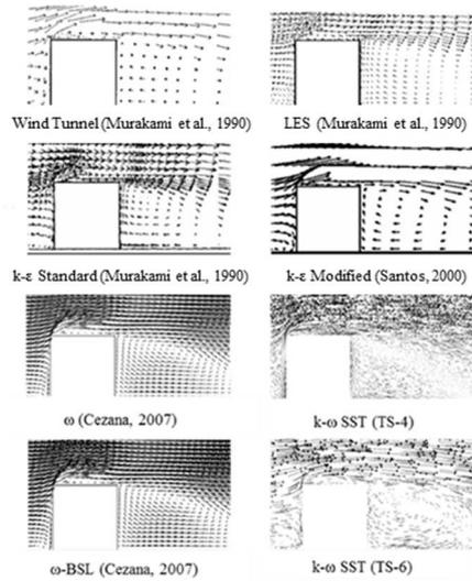
Figure 5. Vector field in plane of symmetry.
