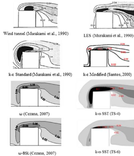
Figure 6. Turbulent kinetic energy contour in vertical plane  $xz$  at  $y=(0.0)$ .
