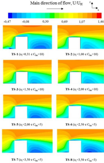
**Figure 3.** longitudinal velocity contour in vertical plane  $xz$  at  $y=(0.0)$ .
