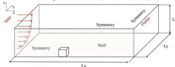
**Figure 1.** Schematic representation of the computational domain and boundary conditions
