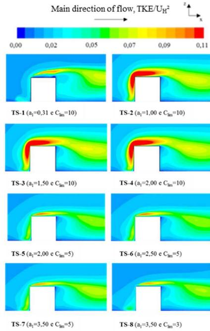
**Figure 4.** Turbulent kinetic energy contour in vertical plane  $xz$  at  $y=(0.0)$ .
