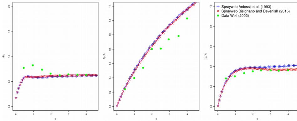
**Figure 1.** Comparison of the measured (Weil et al. 2002) and simulated (both with Anfossi et al. (1993) and Bisignano and Devenish (2015) plume rises) mean height, horizontal and vertical standard deviations for  $F_*=0.1$ .
