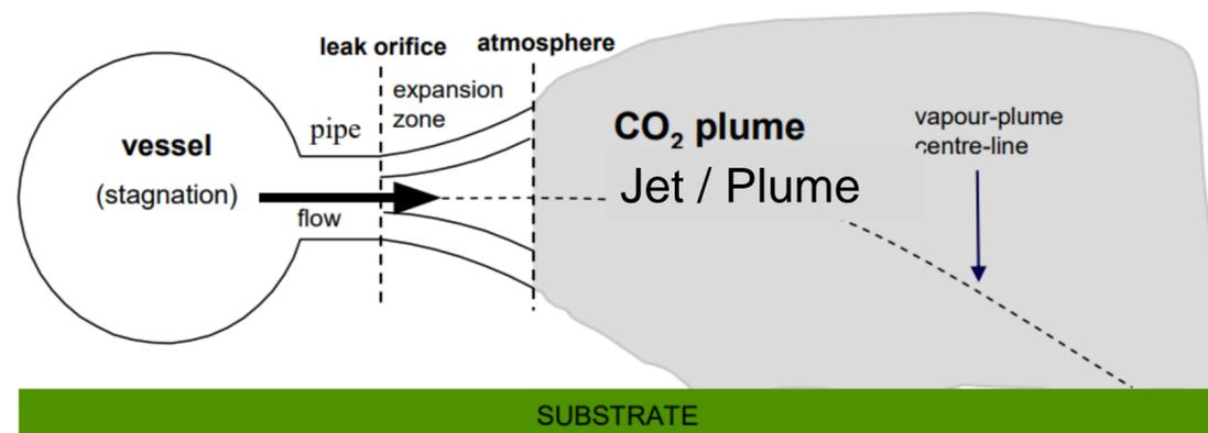
High velocity, low liquid fraction and small droplets (from condensation) all indicate a vapour release was modelled by Phast in these four cases
