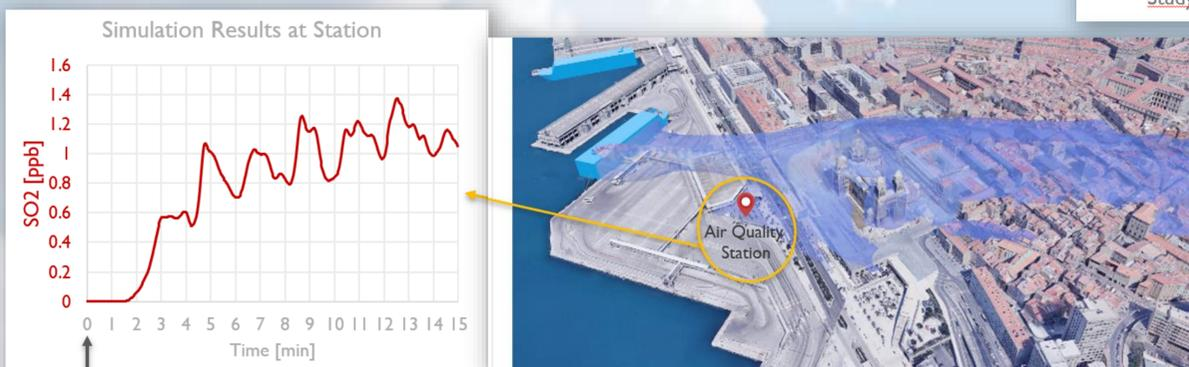
Figure 3: Time-series of SO<sub>2</sub> simulated concentrations with the CFD model at La Major measurement observation site
