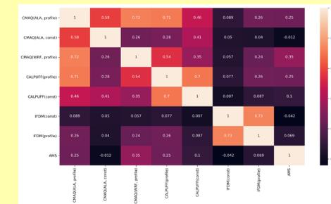
Fig. 8. Correlations between concentrations time series of different models and measured conc. (AMS) at the AMS place.
