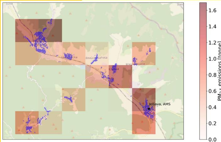
Fig. 1. Red squares:  $PM_{2.5}$  emissions for January in CMAQ model. Blue raster: distribution of  $PM_{2.5}$  emissions to the IFDM and CALPUFF models (the emission flux is not shown).
