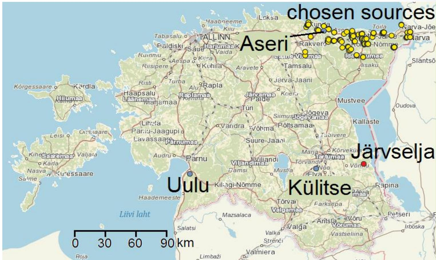
Järvselja mast marked in **red**, lower masts in **blue** (used to estimate inversion geographical extent) and initially chosen industrial pollution sources (stacks) in **yellow**. In the calculations only sources with emission more than 1 g/s were used.
