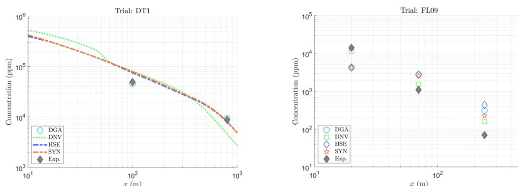
**Figure 2.** Concentration vs. distance plots for the DT1 (left) and FL09 (right) trials.
