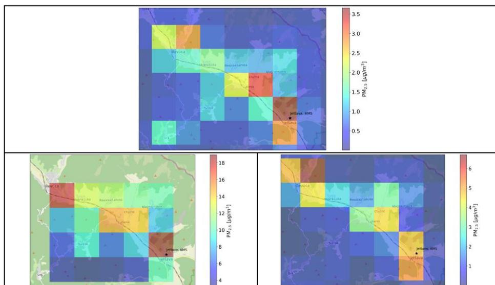
**Figure 4.** Mean PM<sub>2.5</sub> concentrations from residential heating in January calculated by CMAQ model (top). PM<sub>2.5</sub> concentrations resampled to the CMAQ resolution: a) CALPUFF model (bottom left); b) IFDM model (bottom right)
