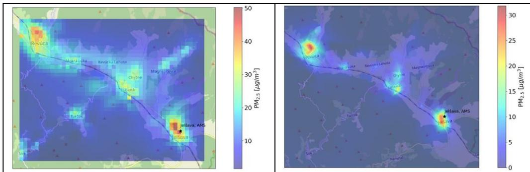
**Figure 3.** Mean PM<sub>2.5</sub> concentrations from residential heating in January 2021 calculated by a) CALPUFF model (left panel); b) IFDM model (right panel)
