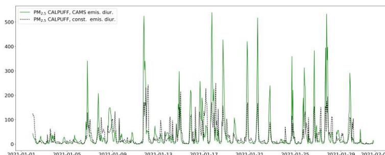
**Figure 6.** Calpuff hourly PM<sub>2.5</sub> concentrations with constant and CAMS diurnal emission profiles at Jelšava monitoring station.
