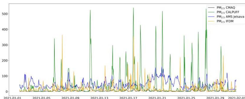
**Figure 5.** Hourly PM<sub>2.5</sub> concentrations at Jelšava monitoring station – models and measurements.
