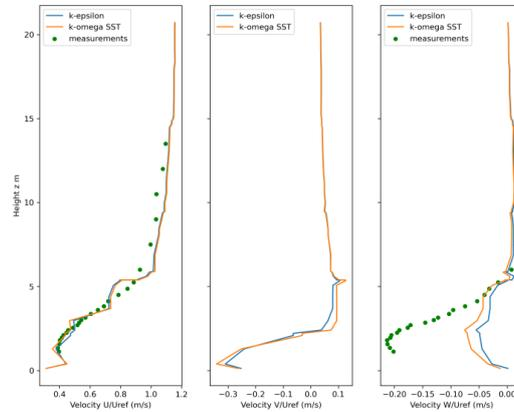
**Figure 2.** Comparison between modeled and measured velocity components profile ( $u/u_{ref}$ ,  $v/v_{ref}$ ,  $w/w_{ref}$ ) at  $x = -109.95$  m and  $y = 0.825$  m
