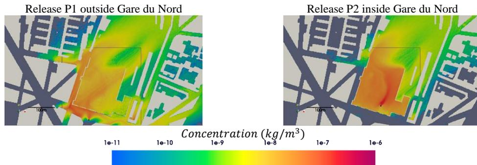
**Figure 5:** Dispersion modeling of releases P1 and P2 in a nested PSPRAY simulation. Positions P1 and P2 are marked by the black dot.
