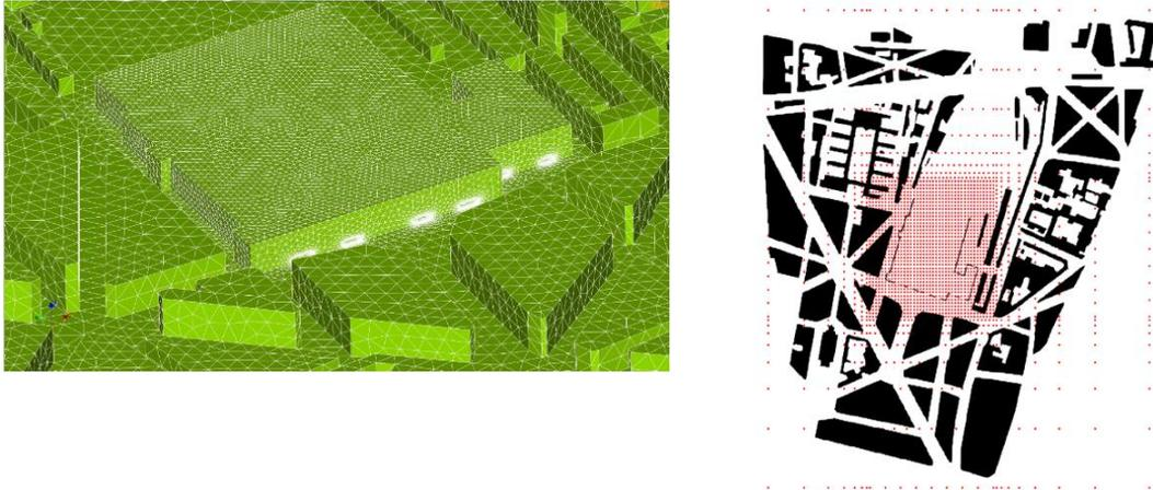
**Figure 2:** Simplified 3D geometry around Gare du Nord and 3D unstructured mesh generated with SALOME (left). Horizontal locations of vertical profiles extracted from the Code\_Saturne simulation (right).
