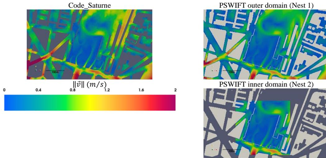
**Figure 3:** Velocity field comparison between Code\_Saturne and PSWIFT at 2m above ground.
