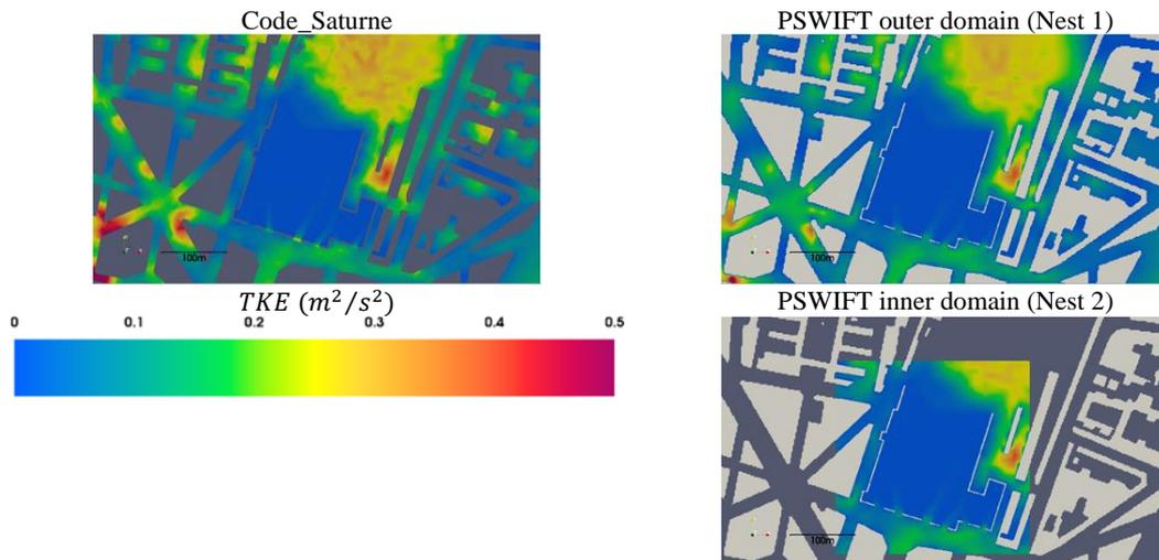
**Figure 4:** TKE field comparison between Code\_Saturne and PSWIFT at 2m above ground.
