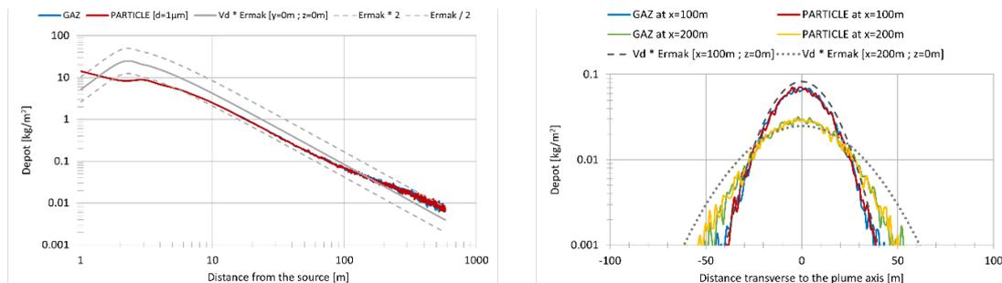
**Figure 4:** Dry deposition along the plume and along the transverse axis for a gas and solid particles with  $d=1\mu m$  for PSPRAY (new mechanism) and the Ermak (1977) Gaussian model
