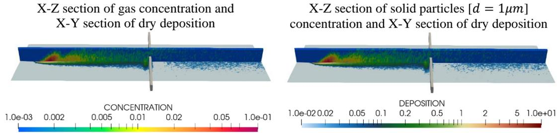
**Figure 6:** illustration of the impact of a building on concentration and deposition
