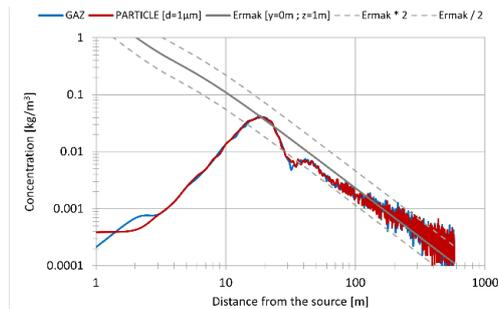
**Figure 3:** Concentration along the plume for PSPRAY and the Ermak (1977) Gaussian model
