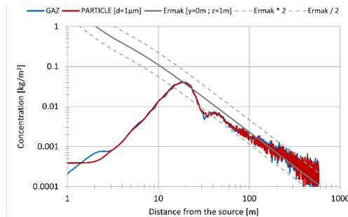
**Figure 3:** Concentration along the plume for PSPRAY and the Ermak (1977) Gaussian model
