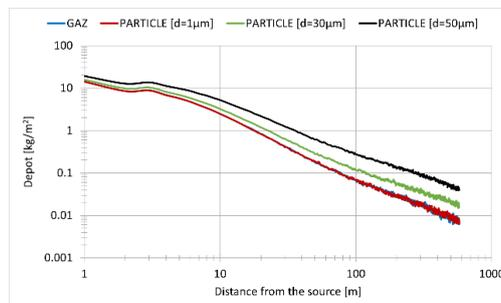
**Figure 5:** Dry deposition along the plume for a gas and solid particles with different diameters (new mechanism).
