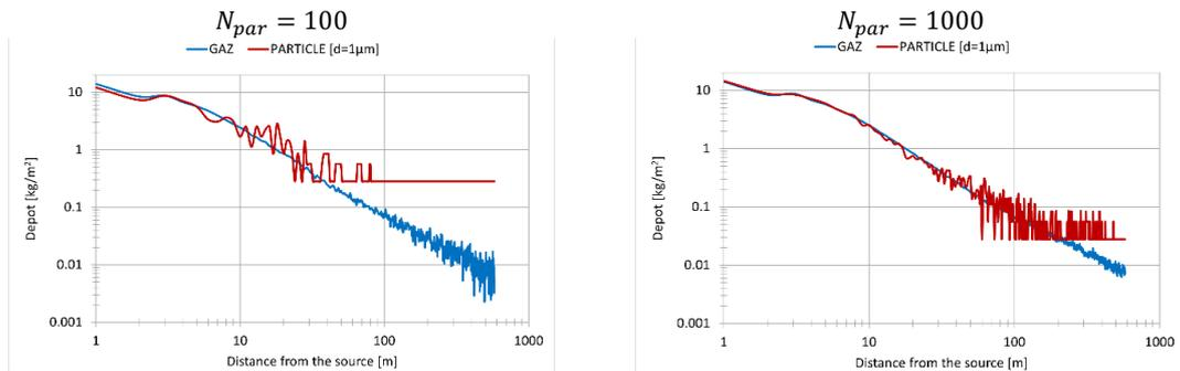
**Figure 2:** Dry deposition along the plume for a gas and solid particles with  $d=1\mu m$  (old mechanism)
