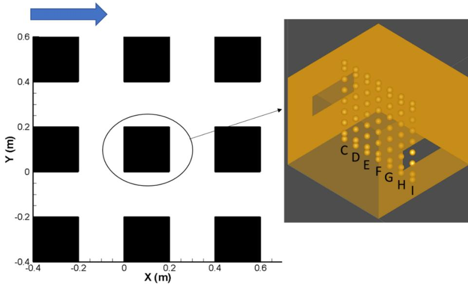
**Figure 1.** Urban model of idealized complexity mounted in the boundary-layer wind tunnel and close-up view of the interior of the target building. The 63 sensors inside the target building are presented also (yellow circles).
