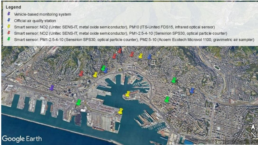
**Figure 1.** Monitoring network around the port of Genoa (Google Earth Pro V 7.3.4.8642)
