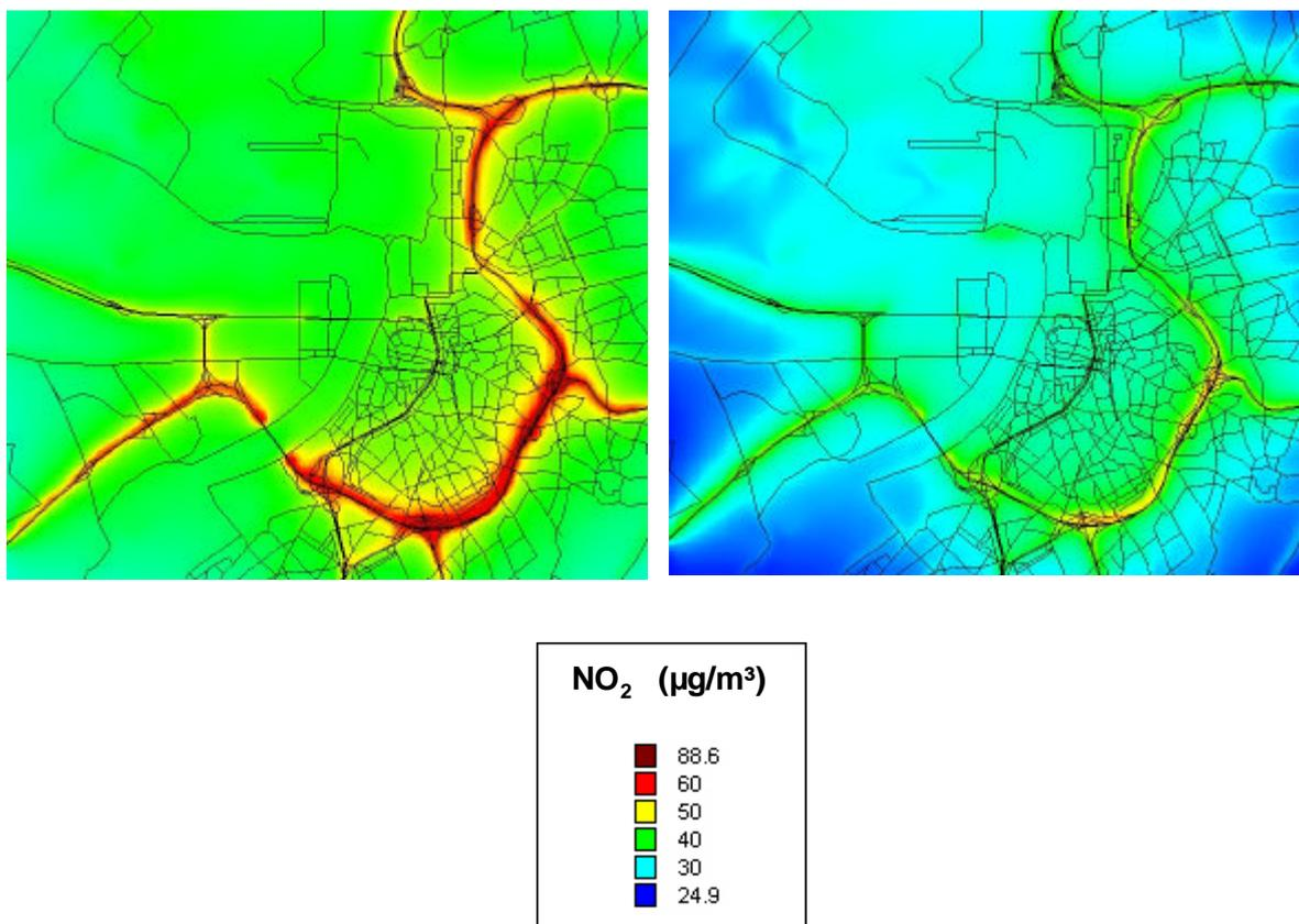
Figure 3. Calculated annual NO<sub>2</sub> concentrations for the reference case in 2003 (left panel) and the situation in 2015 after implementation of the tunnel scenario (right panel).
