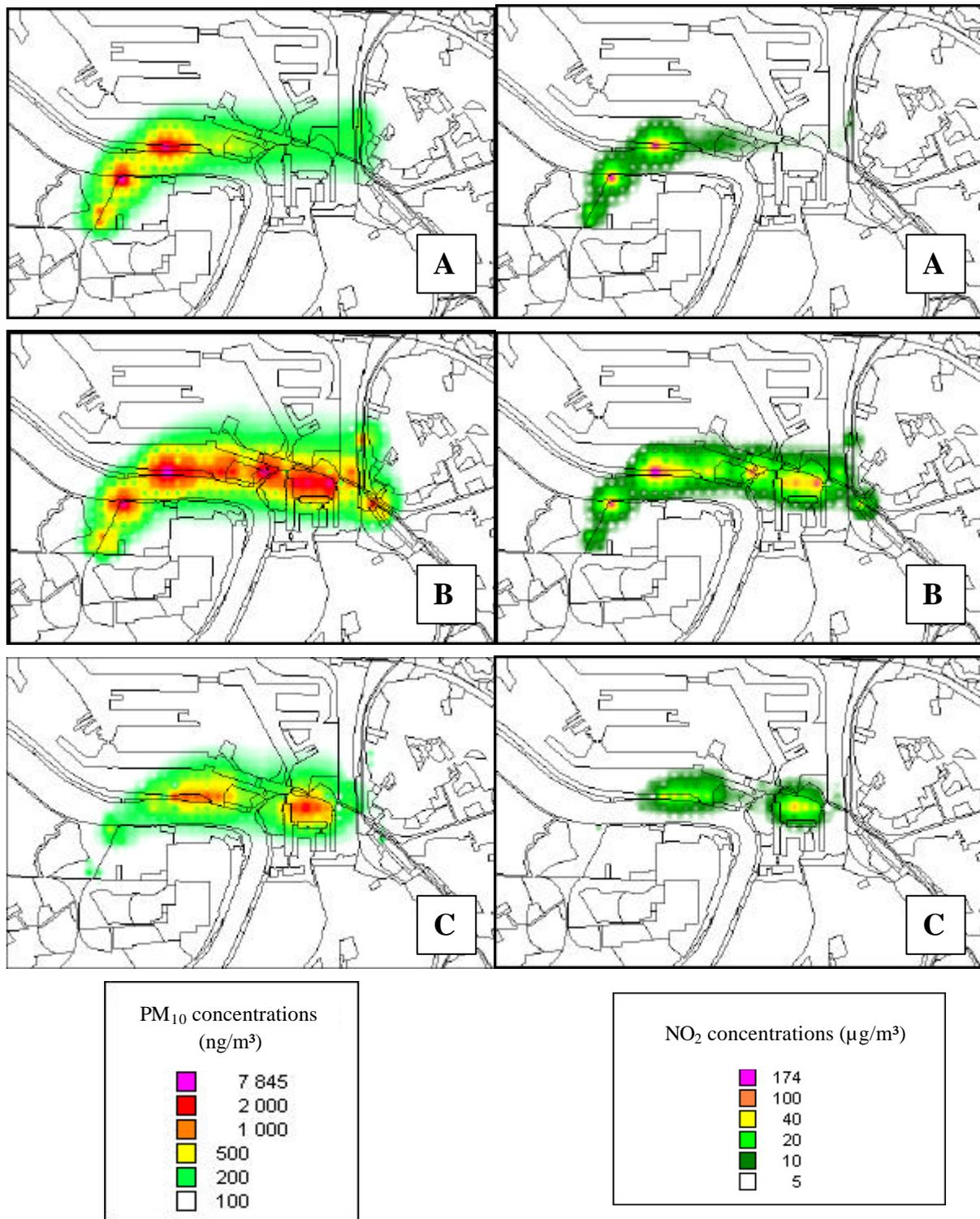
Figure 2. Calculated increase in annual PM<sub>10</sub> concentrations (left panels) and annual NO<sub>2</sub> concentrations (right panels) for A) the viaduct scenario; B) the tunnel scenario with exhaust height of 5 m. and C) the tunnel scenario with exhaust height of 30 m.
